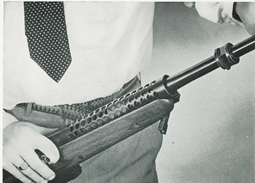
Fig. 5 —Withdrawing the barrel from the receiver after releasing the barrel latch assembly. Operating handle is raised by the right forefinger to unlock the bolt from the barrel.
