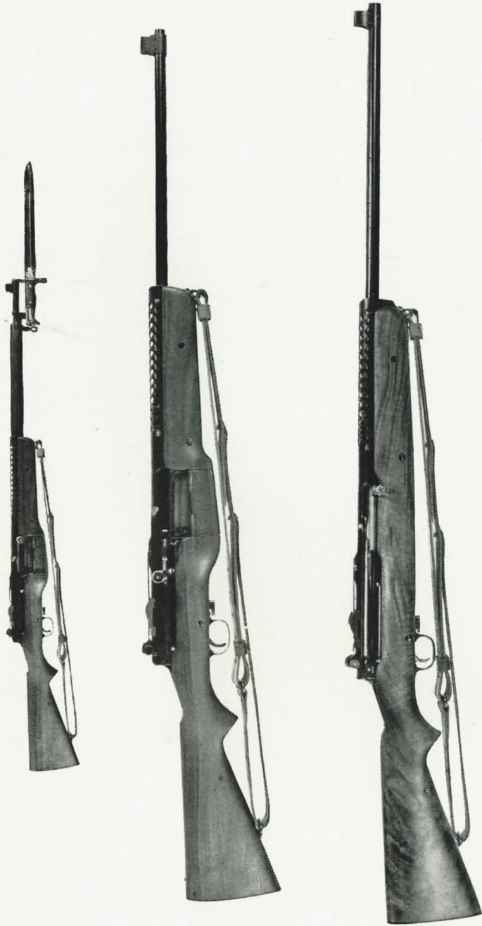
Top—Johnson Semi-Automatic Rifle, Type R, with 10-shot rotary feed magazine, bayonet and handguards attached. Center—Johnson Semi-Automatic Rifle, Type R, with 10 shot rotary feed magazine. Bolt is shown open, as it remains after the last shot is fired. Bottom—Johnson Semi-Automatic Rifle, Type V, with detachable box vertical feed magazine.
