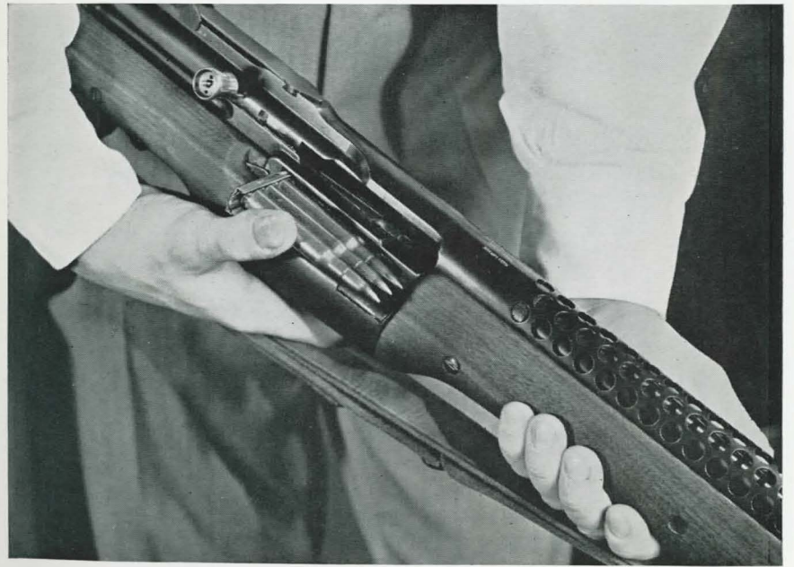
Fig. 2—Charging the 10-shot rotary magazine from a Springfield clip—bolt open.
