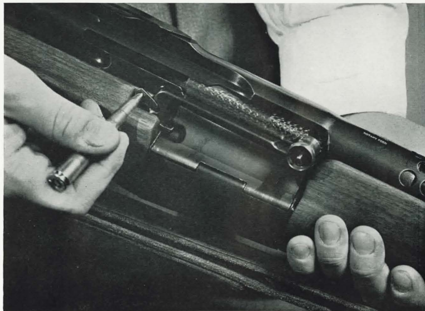
Fig. 10 —Disengaging the hammer block pin with the point of a cartridge. The hammer block pin is then withdrawn.
