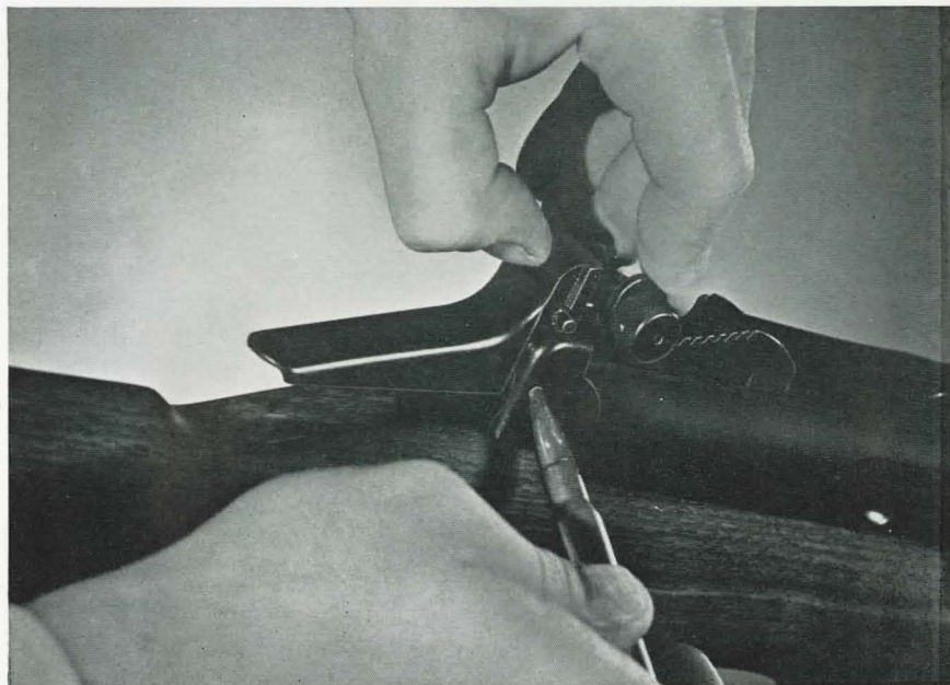
Fig. 6 —Removing the bolt stop plate after having disengaged the bolt stop plate plunger by depressing it with the point of a cartridge.
