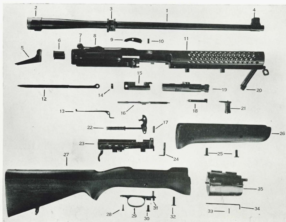
Fig. 13—Johnson Semi-Automatic Rifle, Type R, completely stripped.
