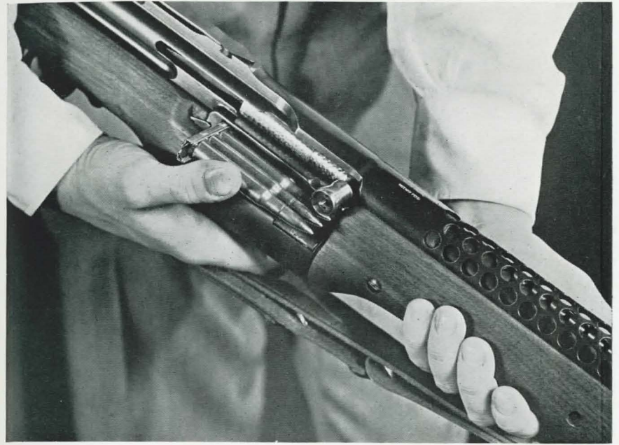
Fig. 1—Charging the 10-shot rotary magazine from a Springfield clip—bolt closed.
