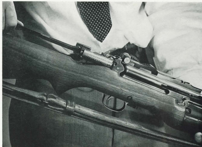
Fig. 9 —Withdrawing the bolt group from the receiver after having removed the operating handle.
