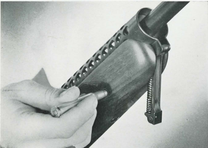
Fig. 4 —Dismounting the barrel. The barrel latch plunger has just been disengaged by the point of a cartridge and the barrel recoil spring and latch assembly has been swung out of its locked position by recoiling the barrel manually with the left hand.
