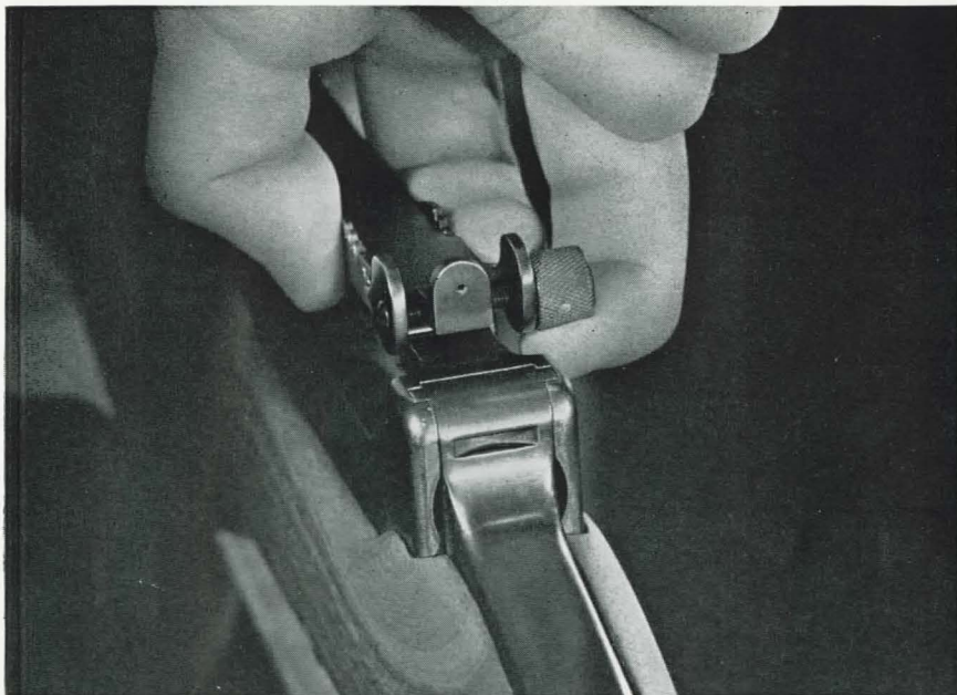
Fig. 3 —Elevating the rear sight by sliding the rear sight elevator to the rear with the thumb and forefinger while lifting up on the windage knob to raise the rear sight leaf.
